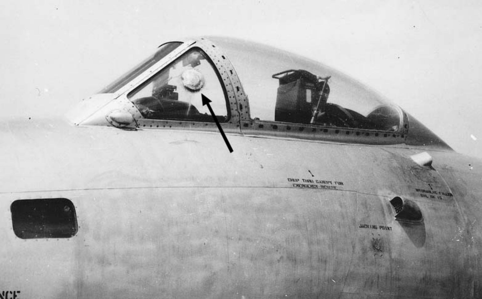
Charanjit Singh's Canberra IF 898 after local repairs to windscreen day after hit by ground fire; back to flying
